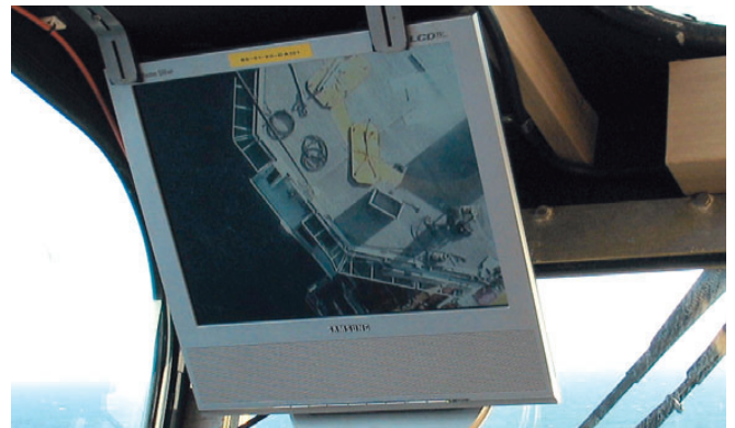
The crane camera is installed to overlook the topside of the load and crane hook assembly, enabling the crane operator to manoeuvre the load safely and efficiently via detailed images relayed to his monitor.
