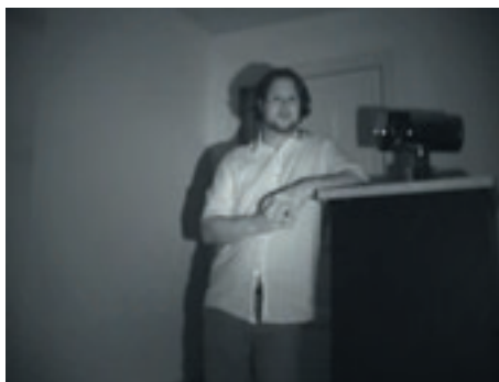
Picture taken with Day/Night CCD Camera with IR Light directed at the target (Near IR – light invisible to the eye)
